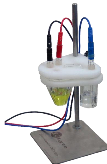
Figure 3.2. Electrochemical cell setup
