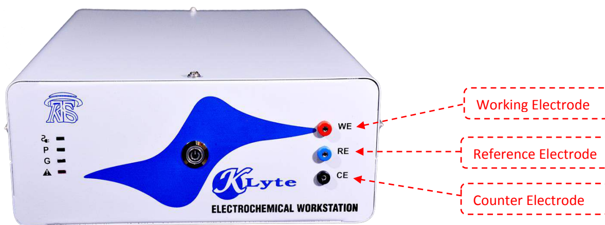
Figure 5.1 – Connector sockets for Working, Reference and Counter Electrodes
